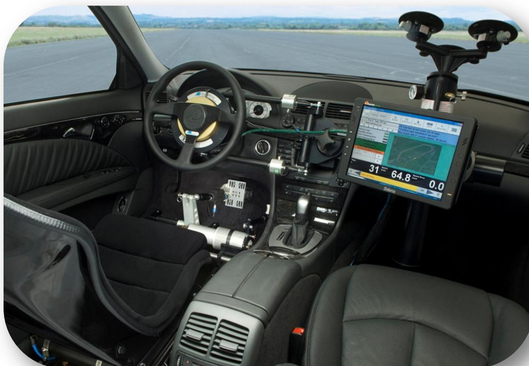
The SR30 steering robot, BR1000 brake robot and AR1 accelerator robot (configured here for the Driverless Test System)
