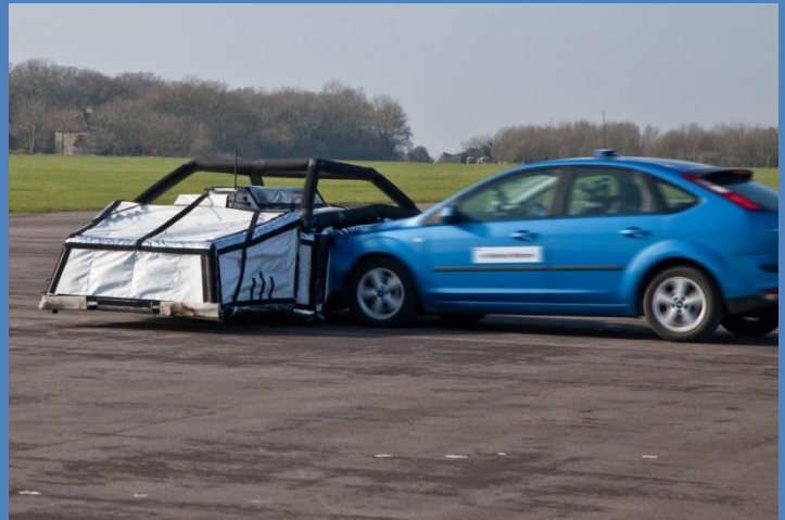
Side impact (both vehicles moving at 30km/h)
