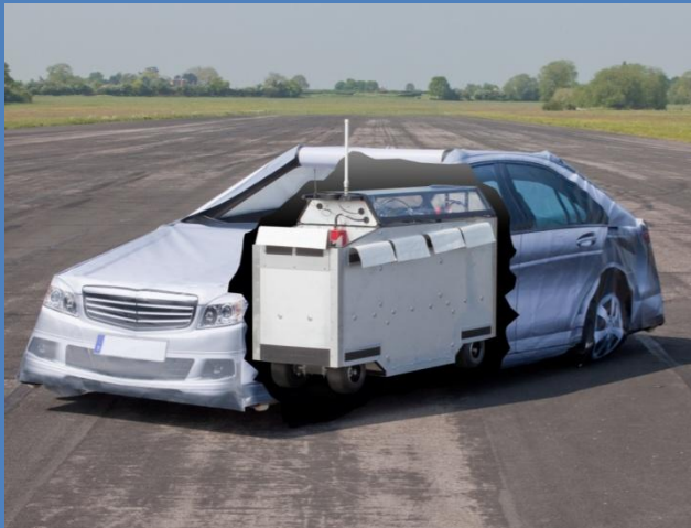
Cut-away showing central drive box inside SCTV cushions
